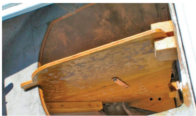
This rode locker partition breaks down into two pieces and can be quickly removed to improve access to the windlass motor and other vital items inside
