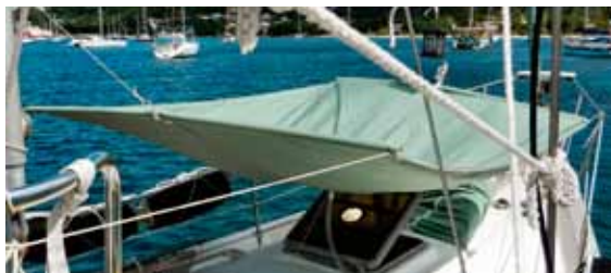
A small foredeck awning configured to catch rain is an easy way to augment your water supply
