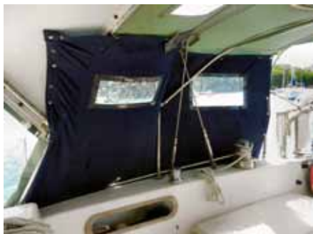
A simple fabric curtain that you can switch from one side of the cockpit to the other will help keep you dry when the spray is flying
